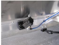
Vibra-Might VMR 1125 and VMR 1200 vibrators attach to trailer knock rails and generate 5,000 and 3,000 vibrations per minute, respectively.
