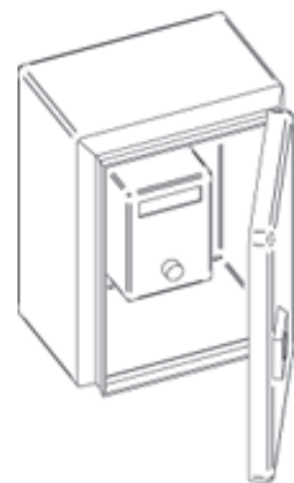
SIC Control Package Required for SI vibrators. One-second timer standard, additional time cycles available.
