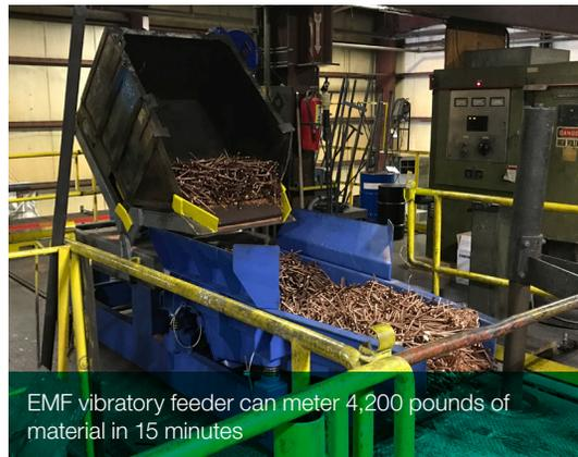
EMF vibratory feeder can meter 4,200 pounds of material in 15 minutes
