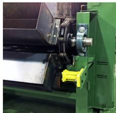
Material at the unloading station is completely knocked out of the bins by a CVC 1200 VMRAC extended piston (EP) air-cushioned pneumatic vibrator.
