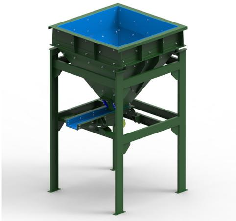
**Bed depth of material on the tray.** The material must be free flowing and always available in the hopper to charge the feeder. Not enough material will “starve” the feeder, reduce the bed depth, and cause inconsistent discharge rates.
