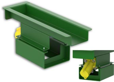
*Air-powered Feeders* work best under hazardous conditions because they are driven by an air-cushioned piston vibrator, which produces smooth linear force and can work safely in high temperatures. It is the simplest of the three feeders to maintain and the controls are the most economical.
