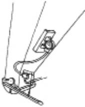
Synchronize the action of your vibrator with the opening and closing of the gate by mounting a CVC JN quick acting valve near the gate handle. Connect the JN handle and gate handle with cable and spring illustration as illustrated. When gate handle is pulled, the vibrator will start automatically to ensure flow of material.
