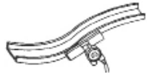
No need to experience clogging or material slowdown on chutes of a curved configuration. Simply weld a piece of 'T' or 'L' iron to the side of the chute at the trouble spot and bolt on an appropriately sized vibrator.
