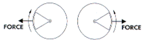
Figure 2 - both eccentrics outward and opposed, 180° apart. Resultant force is due to cancellation effect.
