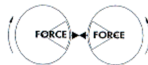
Figure 4 - Both eccentrics inward and opposed, 180° apart. Resultant force is zero due to cancellation effect.
