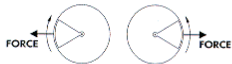
Figure 2 - both eccentrics outward and opposed, 180° apart. Resultant force is due to cancellation effect.
